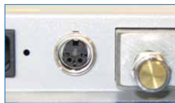
The Signalization plug is used to connect to a remote location such as a control room.
