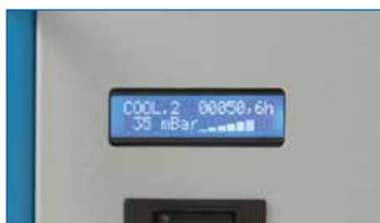
Digital readout indicates the pressure in digital and analog forms as well as the operating time and process.
