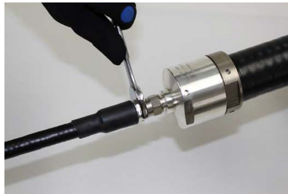
Step 2 - With an open ended wrench hold connector body in a fixed position
