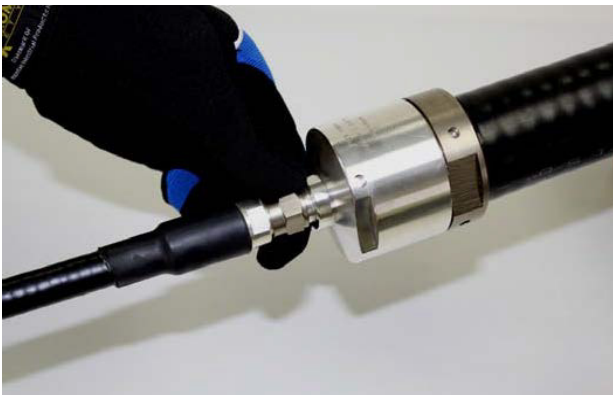
Step 1 - Attach coupler nut finger tight
